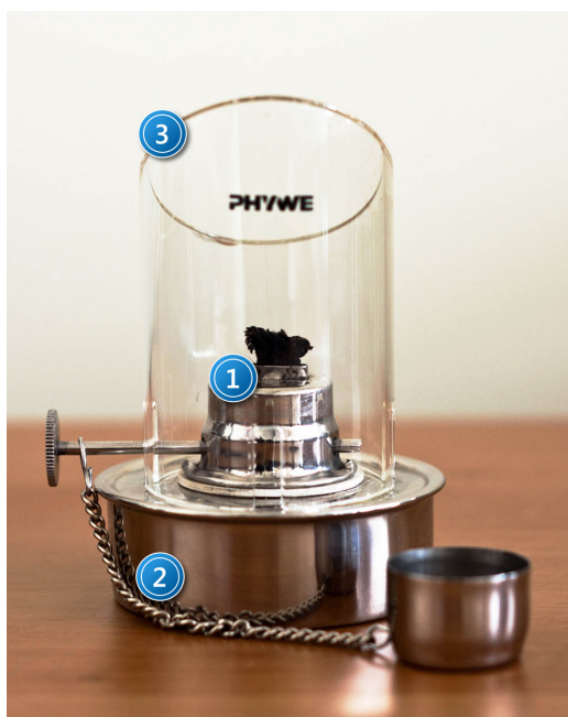
Picture 3. View of the burner: 1 – screw-cap; 2 - container; 3 - chimney.
