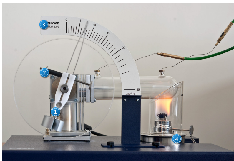
Picture 2. Operating Stirling engine: 1 – torque-meter; 2 – adjustment screw; 3 – measuring scale; 4 – burner with chimney.
